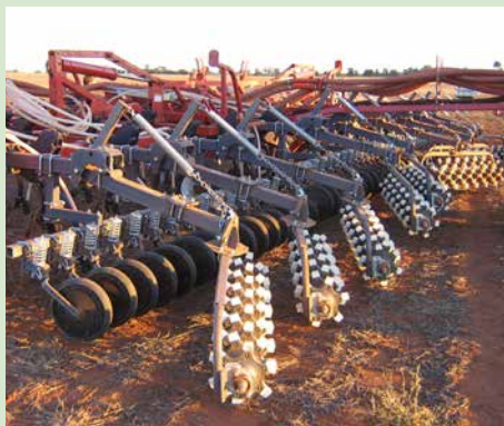
Presswheels and harrows combination
