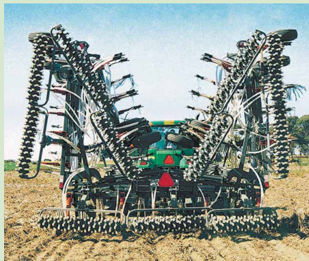
Double fold machine with star harrows
