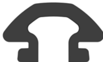
70mm 'V' Tyre General purpose in mixed soil types 40-85mm Closers or Seekers PWV70 $450 +GST
