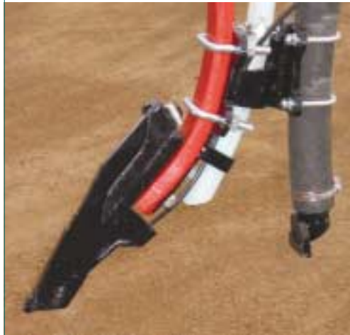
Modified point for liquid fertilizer
